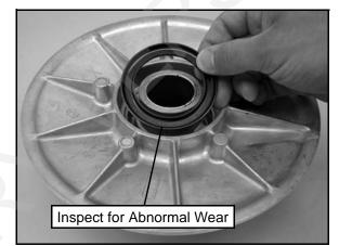
8. Check the rollers in the stationary sheave for wear. If rollers are worn, a new driven clutch assembly may be needed.
