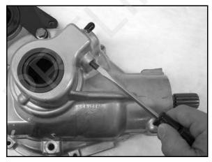
18. Carefully remove the shift yoke assembly from the gearcase cover.
