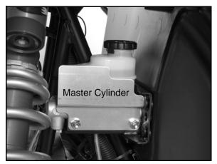
2. Remove the clip (A) from the clevis pin (B) that attaches the master cylinder to the brake pedal lever.
