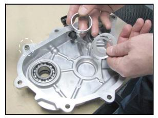
9. Disassemble the cover as required, replacing components that are failed or worn. Check bearings for wear or damage and replace as needed using a press and standard bearing removal tools. *Discard removed bearings as they become damaged by the removal process.*
