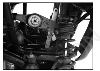
7. Torque the remaining bolt that attaches the bracket to the front side of the rear gearcase.
