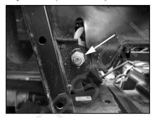
6. Remove the (3) Torx fasteners and (2) push rivets from the rear RH panel divider. Remove the panel divider from the vehicle (see Chapter 5).
