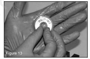
Install a new u-cup seal into bearing assembly (Fig. 14). After installing u-cup seal, install a new o-ring.
