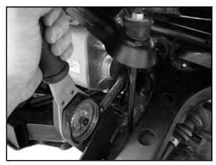
5. Remove the special tool and attach an extension to the torque wrench. Torque the bottom bolt that attaches the bracket to the rear gearcase through the hole in the frame support.
