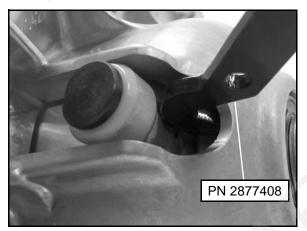
NOTE: Make sure the tool is square with the moveable sheave surface of the driven clutch.
