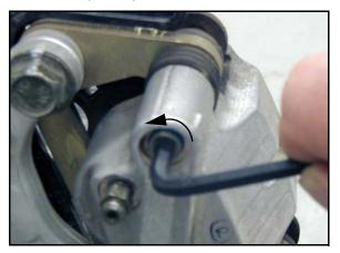
4. Remove the upper and lower caliper mounting bolts and remove the caliper from the front hub.
