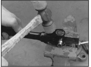
4. Force U-joint cross to one side and lift out of inner yoke.
