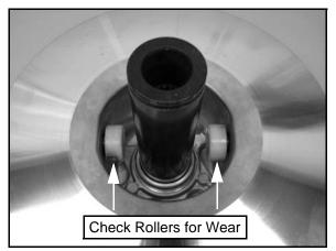
9. Inspect the bearings inside the moveable sheave.
