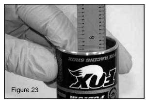
17. Handle the shock body with care after setting the IFP depth. Do not move the IFP after initial setting is established.
