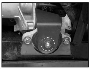
45. Remove the (2) lower bolts that retain the LH transmission mount to the frame.
