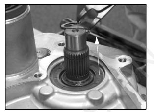
16. Remove the intermediate shaft seal using a seal puller or other suitable method.
