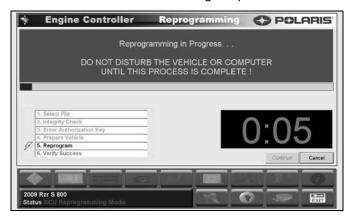
15. Once the ECU reprogramming procedure is complete, click the 'Finish' button on the screen. Verify the reflash was a success by starting the vehicle.
