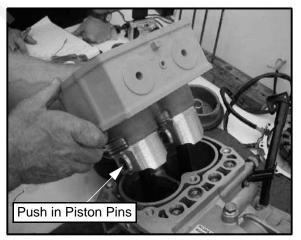
15. Install the piston pin circlips. The circlip ends should be installed at the 12 O'clock position.
