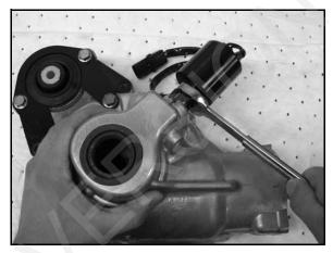
14. If the solenoid was removed for servicing, inspect the tip of the solenoid for wear. If the tip of the solenoid is flattened, the solenoid must be replaced.
