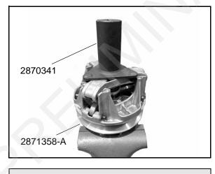
Clutch Holding Fixture: PN 2871358-A Spider Removal Tool: PN 2870341 NOTE: To maintain proper clutch balance and beltto-sheave clearance, be sure to reinstall the original quantity and thickness of washers/spacers beneath the spider during assembly.
