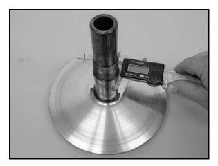
Shaft Diameter: Standard: 1.3745" - 1.375" (34.91 - 34.93 mm) Service Limit: 1.3730" (34.87 mm)
