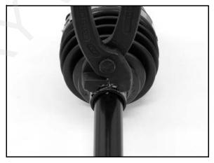
Axle Boot Clamp Tool: PU-48951 or CV Boot Clamp Pliers: 8700226
