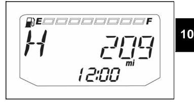
The odometer records and displays the total distance traveled by the vehicle. The odometer can not be reset.
