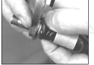
4. Compress the mounting bracket and make sure the dust seals are fully seated. Install the brake pads. Clean the disc and pads with brake parts cleaner or denatured alcohol to remove any dirt, oil or grease.
