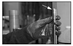
4. Lubricate the shock rod and the Shock Seal Protector Sleeve with new shock oil.
