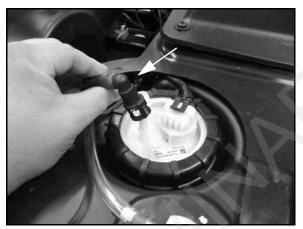
NOTE: A small amount of fuel may come out of the fuel line or tank. Properly drain fuel into a suitable container.
