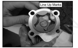
18. Apply assembly lube or oil to the rotors on the oil pump shaft.
