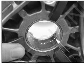
Moveable Sheave Bushing Inspection: Replace the cover bushing if more brass than Teflon™ is visible on the bushing. Refer to bushing replacement in this chapter.
