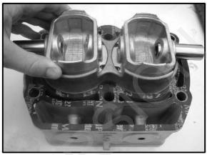
NOTE: To help align the pistons, slide a rod that is close to the same diameter as the wrist pin holes to properly align them in the cylinder.
