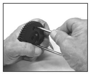
20. After the tapered pins are removed, be sure the cam gear assembly is held together tightly. Place the cam gear assembly on a flat surface. Use the Cam Gear Tooth Alignment Tool (**PU-45497-2**) to align the teeth of the cam gears, as shown in the picture.
