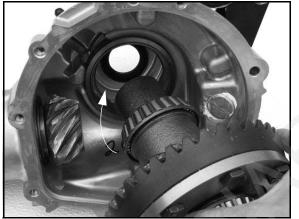
6. Install the gearcase cover. Install the cover screws onto the rear gearcase. Torque to specification.
