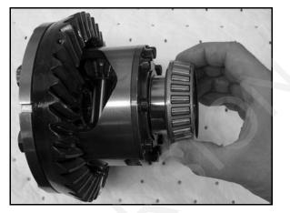
8. Remove the shim(s) from the differential assembly. Be sure to keep the shims together for reassembly.
