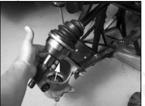
8. Grasp the rear drive shaft and pull sharply outward on the shaft to disengage it from the rear gearcase.
