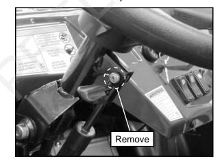
4. Lift the steering wheel up and remove the (2) fasteners that retain the pivot tube.
