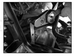
NOTE: A multi-directional torque wrench is required in this application because of the limited access to this bolt. Check with the manufacturer of your torque wrench to see if it can be used to tighten left-hand threaded bolts.
