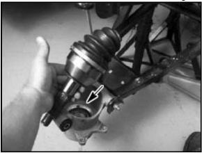
4. Lift bearing carrier into place and install the bolt attaching the bearing carrier to the upper A-arm. Torque fastener to specification.
