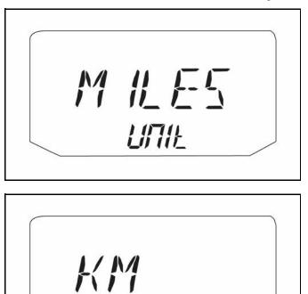
4. Press and hold the MODE button to save the setting
