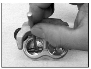
RZR / RZR S: Front Caliper Piston Bore I.D.: Std: 1.004" (25.5 mm) Service Limit: 1.006" (25.55 mm)
