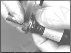
2. Compress mounting bracket and make sure dust boots are fully seated. Install pads with friction material facing each other.
