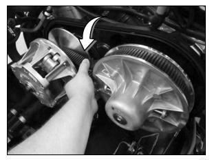
4. Then lift upward on the belt while pulling it out and down over the driven clutch outer sheave.
