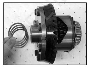
7. Remove the bearing from the lower portion of the differential assembly. Inspect the bearing for smoothness and wear.
