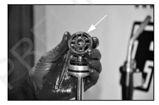
10. Lubricate and install the rebound valve stack.
