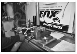
3. Use a spanner or strap wrench to remove the shock body tube and reservoir from the body cap.
