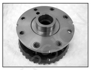
5. Place the differential assembly upright. Use a roll pin punch to remove the roll pin from the differential case.
