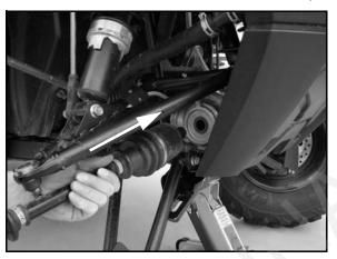
3. Install drive shaft into the front bearing carrier.
