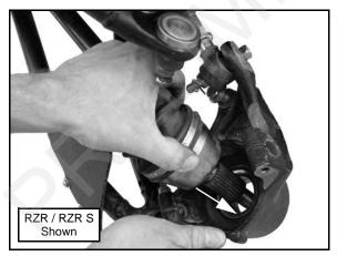
4. Install the upper ball joint end into the front bearing carrier.
