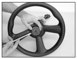
3. Loosen the nut and back it half way off the steering shaft.
