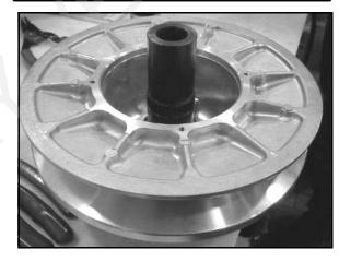
4. Install the roller (A) onto the roller pin (B) on both sides.
