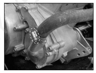
41. Remove the filler neck pressure cap to relieve the cooling system vacuum.
