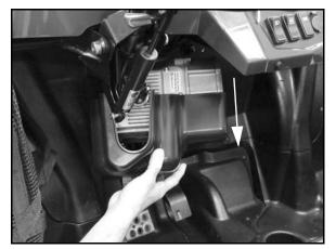
2. Remove the pinch bolt retaining the upper steering shaft to the power steering unit.
