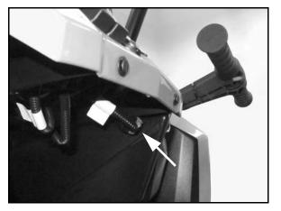
Follow these steps to connect the diagnostic interface cable to the vehicle to allow Digital Wrench<sup>™</sup> use:
