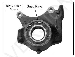
2. From the back side of the bearing carrier, tap on the outer bearing race with a drift punch in the reliefs as shown.
