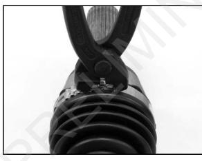
Axle Boot Clamp Tool: PU-48951 or CV Boot Clamp Pliers: 8700226 19. While pulling out on the CV shaft, slide a straight Oring pick or a small slotted screw driver between the small end of the boot and the shaft. This will allow the air pressure to equalize in the CV boot in the position that the joint will spend most of its life. Before you remove your instrument, be sure the small end of the boot is in its correct location on the shaft.
