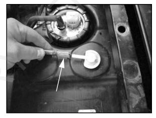
11. While holding a shop towel over the fuel line connector, disconnect the quick connect fuel line from the fuel pump. Move the fuel line out of the way for tank removal.
