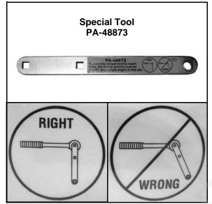
This tool is specifically designed to access the critical transmission to rear gearcase mounting bracket bolts on the *RANGER* RZR when the transmission and rear gearcase are installed in the vehicle. This tool allows for proper torque to be applied to ½" SAE hex head cap screws with limited wrench access. When used at a 90° angle with a torque wrench, no torque multiplier is necessary.
