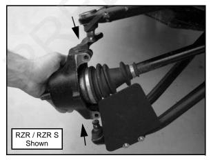
3. Install pinch bolts and torque to specification.
