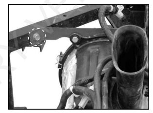
25. Remove the airbox and throttle body from the vehicle as an assembly. Take care in not allowing the throttle cable to bend excessively or kink. Carefully place the assembly on the floor next to the vehicle. Insert a shop towel into the engine intake adaptor to prevent dirt from entering the engine.
