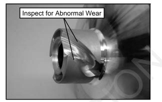
7. Inspect the inner spring retainer for wear and replace as needed.
