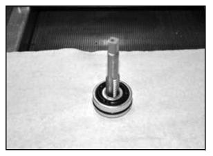
3. Use a large punch to drive out the bearing.
